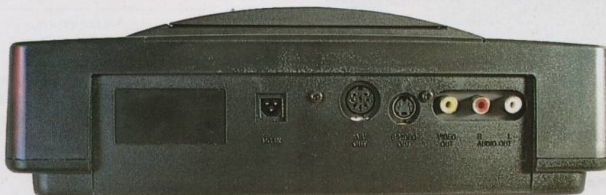
The new joypad (above) has a micro-switched directional control which works well. The rear of the machine features (from left to right) RGB SCART, S-Video, composite video and stereo jacks
