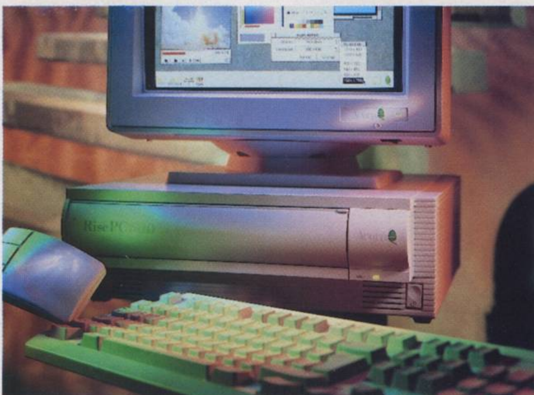
Acorn's RISC PC is based on an ARM610 CPU, a 32bit RISC chip like the PowerPC and the 3DO's central processor (see David Young's letter)
